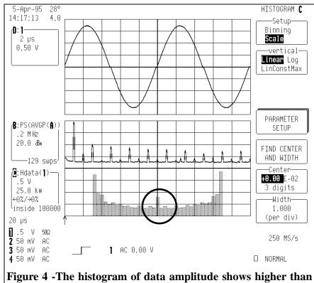
Figure 4 -The histogram of data amplitude shows higher than normal number of sample values at the zero crossing (circled) indicating that the high harmonic levels are due to crossover distortion
