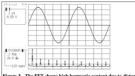
Figure 3 - The FFT shows high harmonic content due to distortion but provides no clues to its source.
