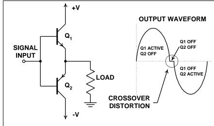
Figure 1 - A simplified view of a push-pull amplifier showing the source of crossover distortion.
